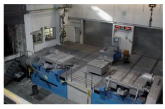
Furnace platform of an MFT Ge 8,000 / 6,000 kW unit
