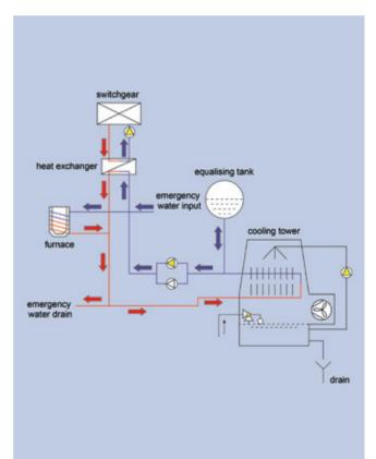
Water recooling system with cooling tower
