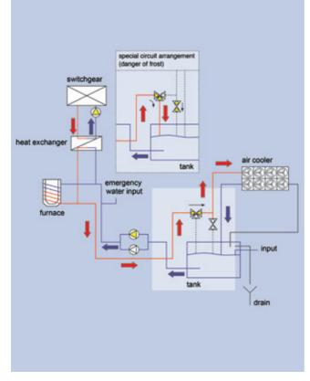
The water recooling system is operated either in normal mode or – at lower outdoor temperatures – in a special operating mode in which the entire air cooler contents is automatically drained into an intermediate tank which closes the cooling circuit.
