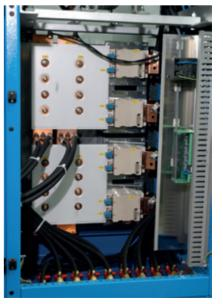
IGBT converter for 3,000 kW
