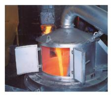
Transfer from melting furnace to holding and pouring unit
