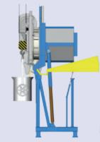
Narrow design for pouring into crane ladle
