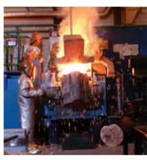
Capacity Power, max. Melting rate, max. (kg) (kW) (kg/h) 500 500 950 750 750 1,400 1,000 1,000 1,900 1,500 1,500 2,850 2,000 2,000 4,000 3,000 3,000 6,000 4,000 4,000 8,000 5,000 5,000 10,000 6,000 6,000 12,000 8,000 8,000 16,000 10,000 10,000 20,000 12,000 12,000 24,000 16,000 14,000 28,000 18,000 16,000 32,000 25,000 20,000 40,000
